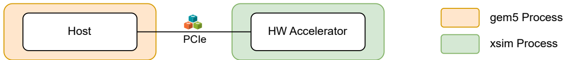
Figure 2.2: The instantiation of the simple heterogeneous system from Figure 2.1 in the full-system simulation framework SimBricks ( ). SimBricks connects the two simulator processes by forwarding requests and responses via shared memory queues and synchronizing the two simulators.
